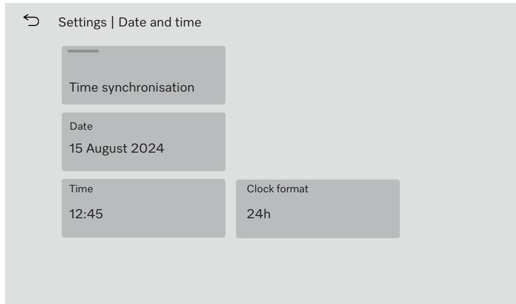
Time synchronisation The date and time can be set using time synchronisation via the internal CKM communication module. (See section “Network connection”, “CKM communication module”.)
