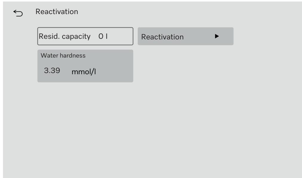
**Remaining capacity** The softener must be reactivated regularly to provide soft water. In the Remaining capacity field, you can see the remaining amount of water available until the next reactivation.
