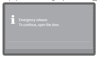
The message is acknowledged when the door is closed.
